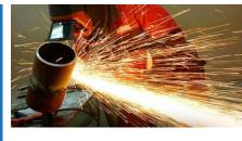
What is HOT WORK? Basically, hot work is any operation or task that produces a flame, heat or sparks such as electric or gas welding, abrasive cutting, soldering, grinding, torch work and brazing activities. This includes torches, arc welding equipment, portable grinders and propane torches. This also includes non-rated electrical tools and equipment when used in a hazardous environment.
